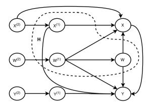
Fig. 3. Example graph depicting the resulted set H when the impact of X on Y is examined. At this example, X precedes temporally Y and W precedes X. The maximum examined time-lag L is 2.
