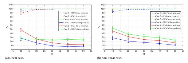
Fig. 5. Comparison of the MDT, CMI and MGC causality detection methods on synthetic data.
